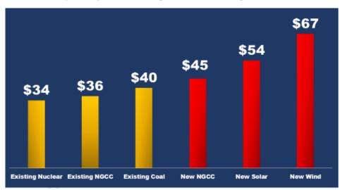
LCOE (\$/MWh) for electricity sources in 2020 per EVA model
